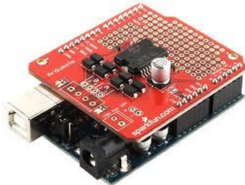
Figure 6: Ardumoto motor shield
